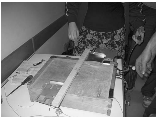
Fig. 9 The rotating scratch machine
